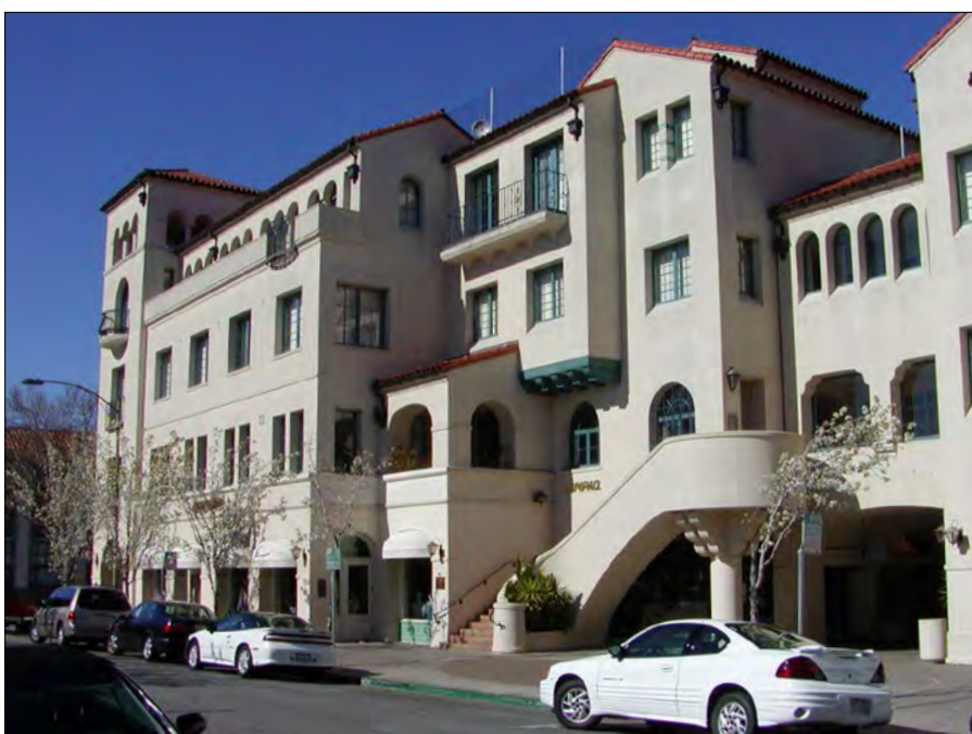
A mixed-use building employs varied massing and pedestrian-oriented elements (awnings, balconies, stairs, doors, and windows) that are proportioned in relation to each other and to the building as a whole.
