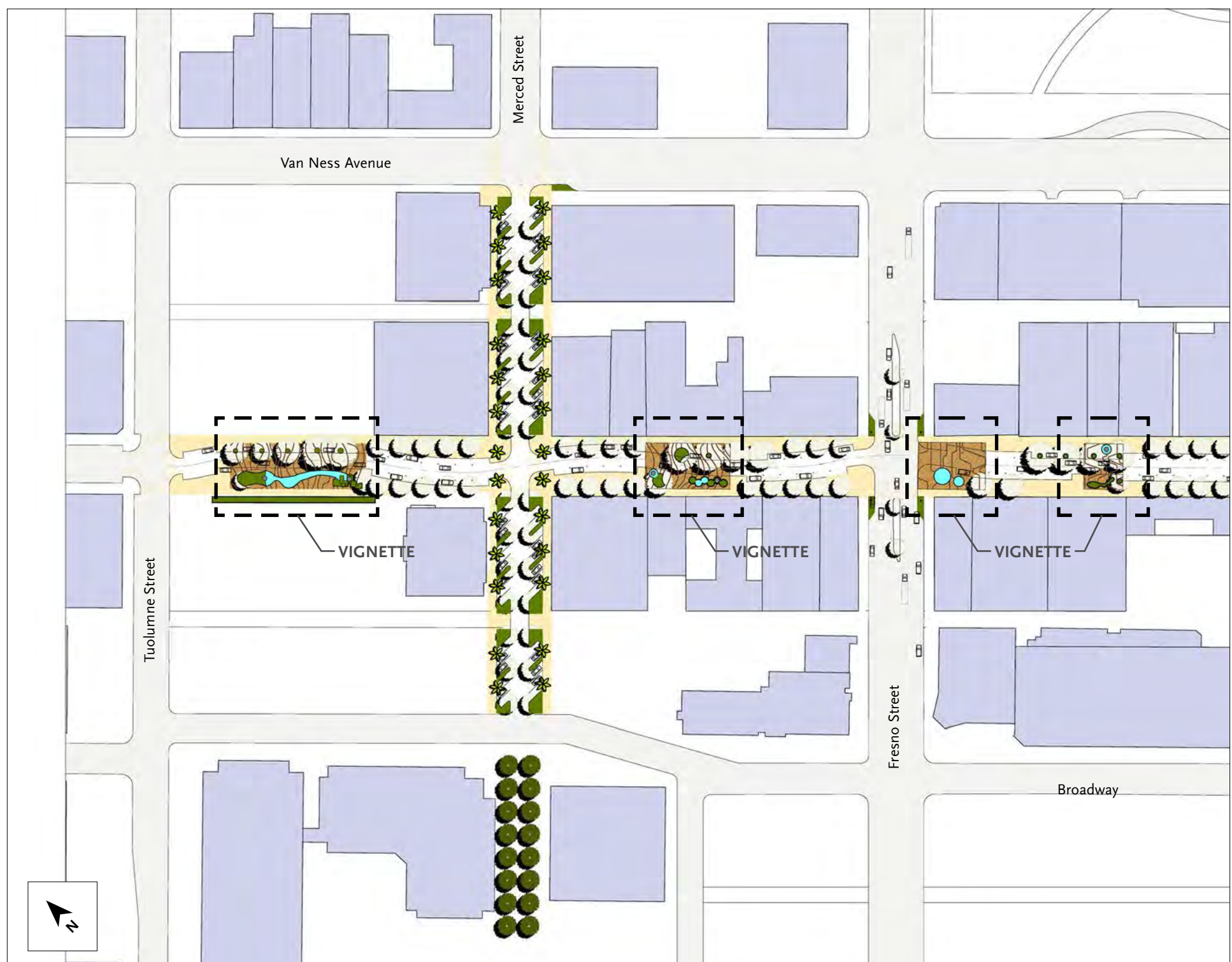
Plan view of Fulton Mall showing an enhanced street that accommodates vehicular traffic winding through selected preserved and renovated portions (“vignettes”) of the original Fulton Mall. The vignettes center around existing fountains, such that most fountains present remain in place and are restored to functionality.
