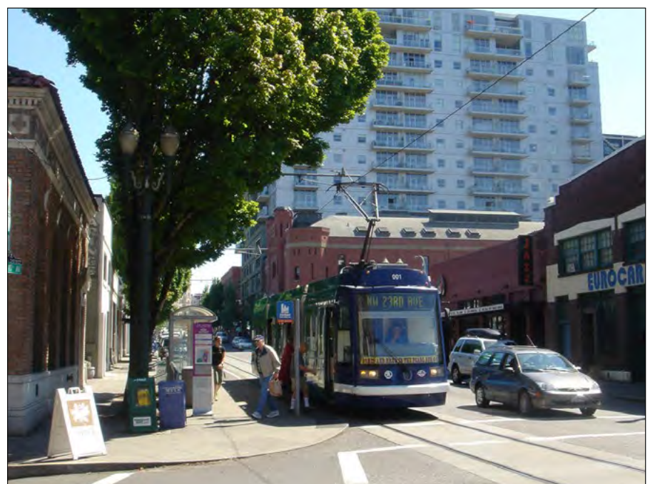
A streetcar shares the road with automobiles and provides ADA accessible access from the sidewalk bulb-out.
