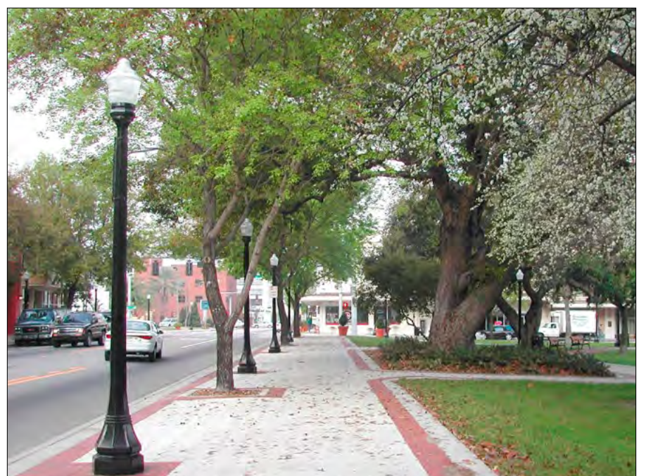
Street lighting is placed away from street trees to give their roots room to grow and to prevent tree limbs from obstructing the lighting.
