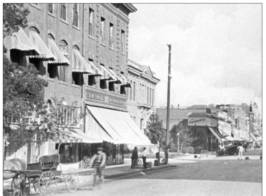
This historic photo of Broadway Street in 1925 shows buildings with ground floor awnings that shade storefront windows and passing pedestrians during hot summers. Upper floor awnings shade upper floor rooms. Credit: San Joaquin Valley Library System
